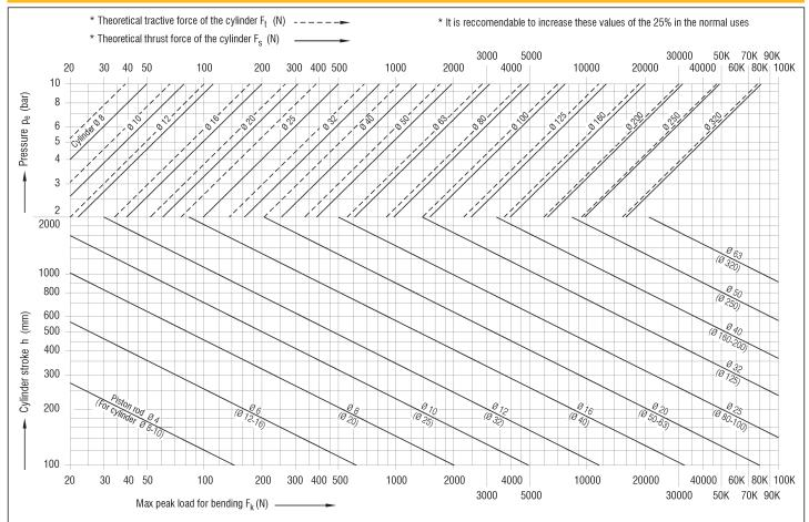
In particular applications the piston rod of the cylinder may be subjected to the peak load; it is then important to control the piston rod diameter in relation to the stroke that should be made, the force developed by the cylinder, the working pressure and the fixings.
