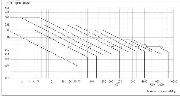
In order not to compromise the correct fuctioning of the cylinders with harmful impacts. it is necessary to cushion the moving mass to gradually reduce its kinetic energy. The maximum absorbable mass depends on the speed of traslation and on the absorption capacity of the pneumatic damper. This diagram gives the speed and the maximum absorbable mass at a pressure of 6 bar for various bores.
